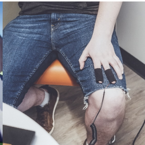
Figure 6. The Galvanic Skin Response (GSR) sensor attached to fingers of a stuttering subject, used to determine stress levels that are used by the ML algorithm.
