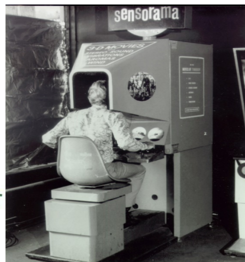
Figure 2. VR: Sensorama, an early VR progenitor. An immersive display with stereoscopic images and stereo sound. Source: scriptanime.wordpress.com
